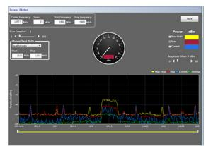
Figure 11: Verify antenna performance using the Power Meter
