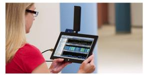
AirMagnet Spectrum ES can scan frequencies between 698 MHz and 2690 MHz and includes support for multiple technologies.
