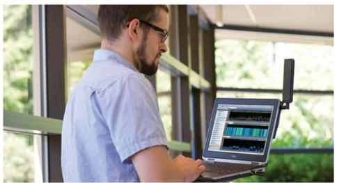
AirMagnet Spectrum ES is a USB-based solution that can be used on any Microsoft® Windows 7 or Windows 8 based Laptop/Tablet PC with a USB port.
