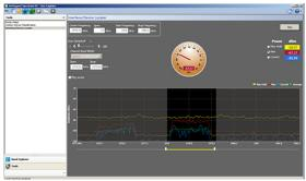
Figure 10: The device locator tool operates as a Geiger counter and beeps louder as users get closer to the interference source.
