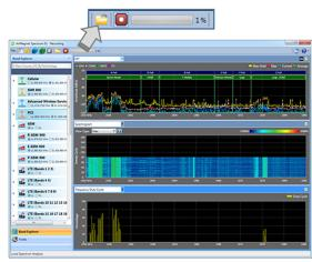
Figure 6: Capture, save and share spectrum trace files for escalations and retaining as forensic evidence.
